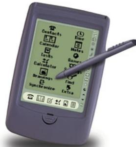
The Palm-size PC user interface supports a keyboard and stylus as input devices. The graphics engine provides support for color and grayscale display devices with up to 32 bits per pixel of color depth, palette management, TrueType and raster fonts, and advanced features such as shape drawing and bit block transfers. The graphics subsystem supports the full UNICODE standard, allowing Windows CE devices to be easily modified for non-United States markets.
